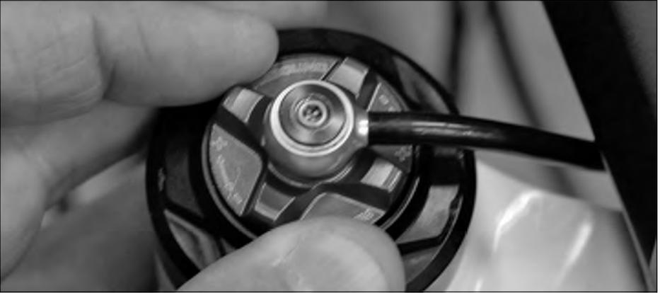
ROTATE DIAL IN THE "--" DIRECTION (COUNTER-CLOCKWISE) TO INCREASE REBOUND SPEED (FASTER).
