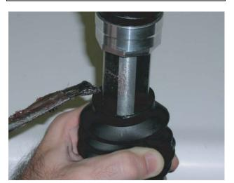
4. Position the boot and secure the boot new zip ties. Make sure the zip ties are installed tightly.
