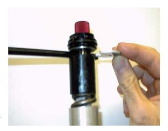
The shims are located between the top washer and preload spacer. Refer to "Illustrations" starting on page 20.
