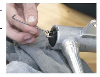
Use a 22mm socket to carefully remove the lower cap. Hold the bottom of the fork up when removing the cap. Once unthreaded, slowly pull up on the cap to remove the compression damper.
