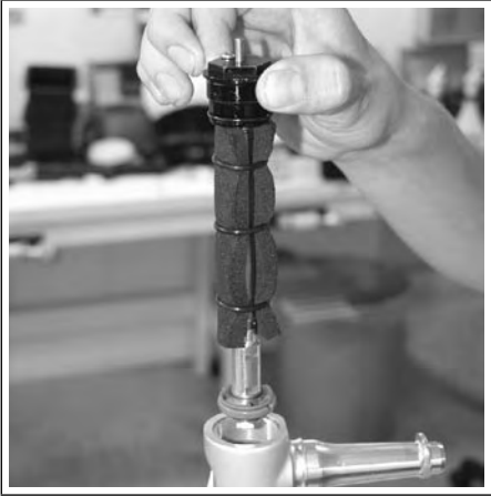
Removing the TPC Damping Assembly
