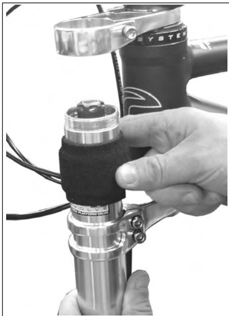
Figure E Lefty Alloy Fork Removal
