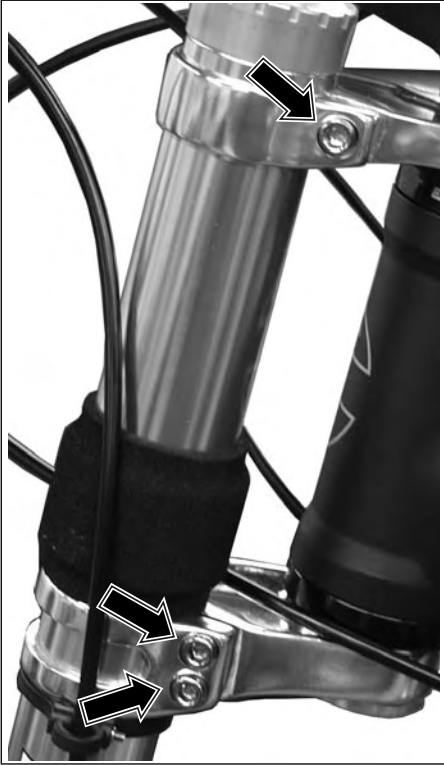
Figure C Lefty Alloy Fork Clamp Bolts
