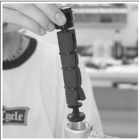
Removing the FFD Damping Assembly
