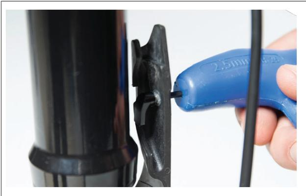
2. Route the brake hose through the channel at the top of the GuideGuard. Rotate the hose clamp so it covers the brake hose. Torque and the hose clamp to 1.5Nm with a 2.5mm hex wrench.
