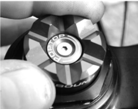
Rotate dial in the “-” direction (counter-clockwise) to increase rebound speed (faster).
