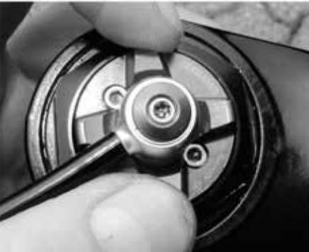
Rotate the red rebound dial in the “-” direction (counter-clockwise) to increase rebound speed (faster).
